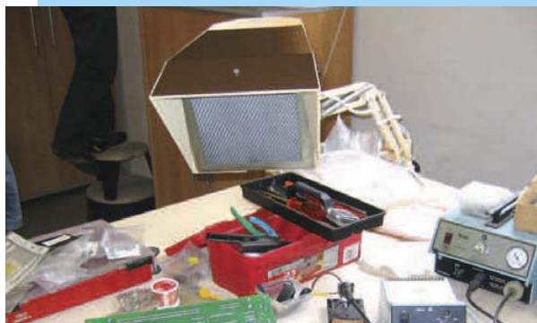
HI 8F filtration mini-hood with an articulated extraction arm
