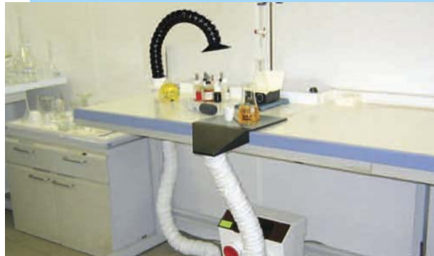
Multi-workstation HI 4P4S in use in a laboratory
